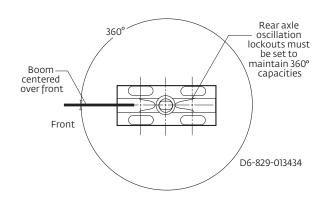
Bold lines determine the limiting position of any load for operation within working areas indicated.
