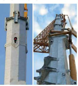
▼ Automatic erection system requires no extra mast section to greatly reduce setup time
